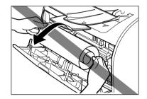
Do not pull the jammed paper upward; the toner on the paper will stain the printer and cause a permanent reduction in print quality.
